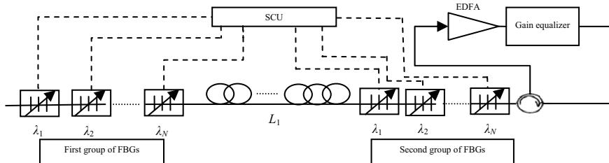
Figure 2. Schematic diagram of the basic building block  $S_{ij}$ .
